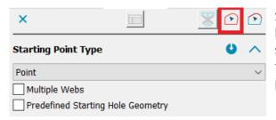
Starting point - defined point: The contour selection button has now been activated. This can be used to select several existing defined starting points in order to change parameters (e.g. the diameter or wire position ...)
